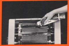
Ink the cylinder with Rex-Rotary quick-drying ink (available in 12 colours).
